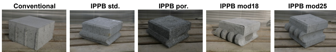
Figure 3. Different types of revetment stones tested in IPPB revetment experiments
