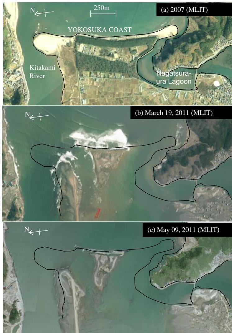
**Figure 7. Aerial photographs of the Kitakami River morphology changes caused by the 2011 Tohoku Tsunami**
