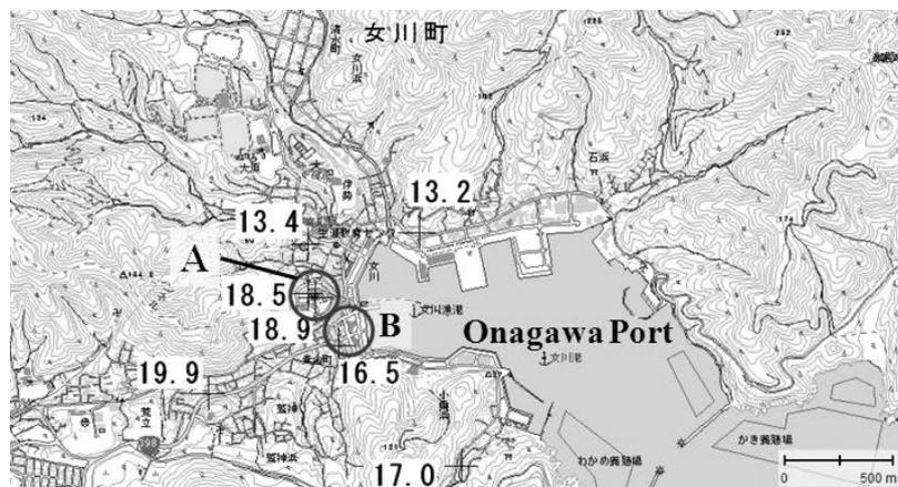
Fig. 9. Distribution of inundation height in Onagawa Town (The unit of inundation height is meter.).
