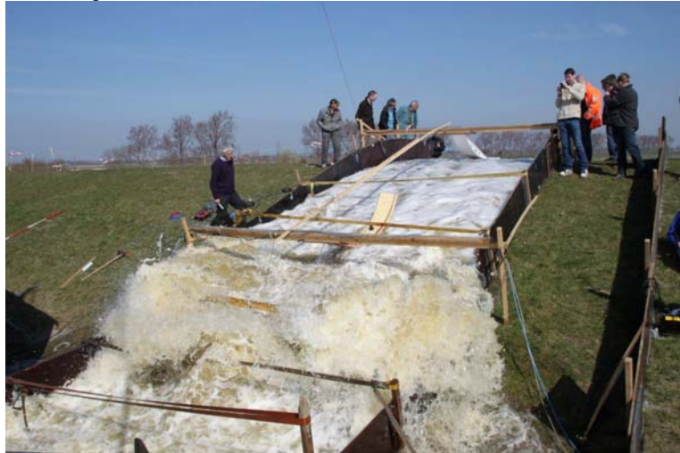
Figure 18. Run-down meeting up-rushing water during the wave run-up simulation process.
