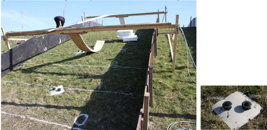
Figure 14. Set-up of hydraulic measurements on run-up with modified surfboard and velocity measurements up and down the slope.
