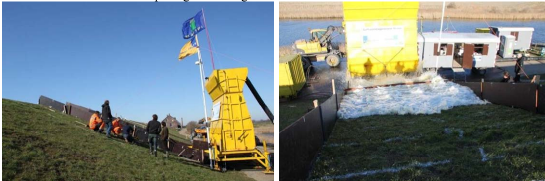
Figure 9. Calibration of run-up levels on a steep slope 1:2.4.
