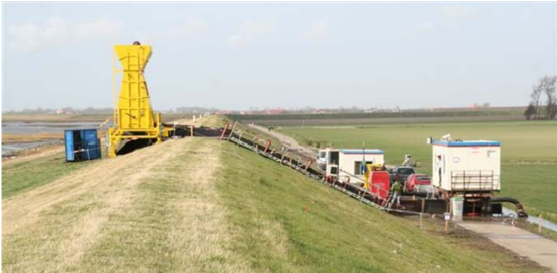
Figure 1. Test set-up of the Wave Overtopping Simulator at a dike.
