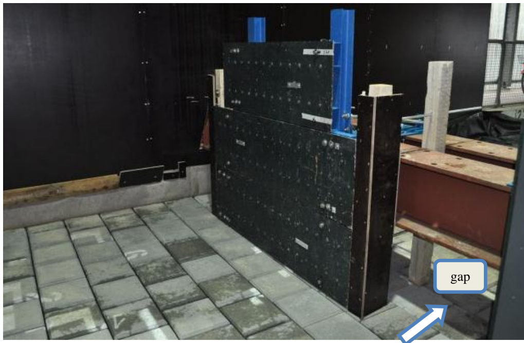
Fig. 6. The left storm wall, flanked by a 10cm wide timber plate for minimizing the side effect.
