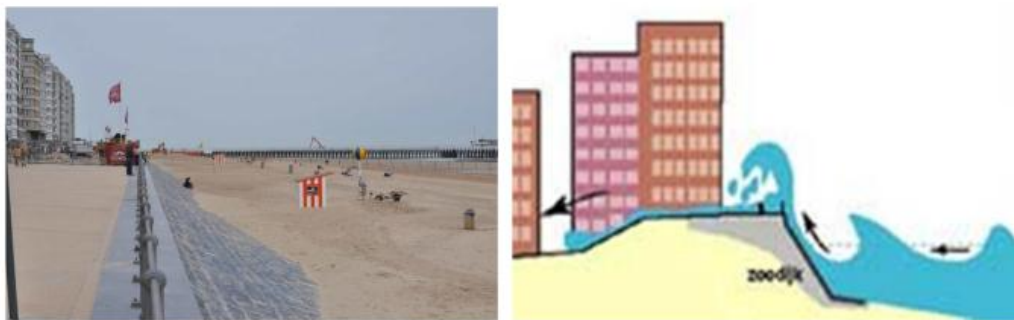
Fig. 1. Typical dike geometry in Belgium, with beach suppletion (left) and without beach suppletion (right)
