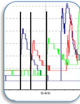
Fig. 8. Time interval between the flow depth recordings, with known distance interval between the sensors
