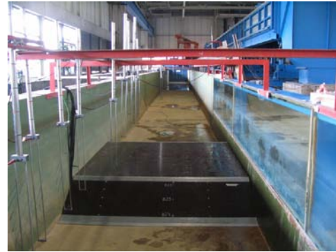
Figure 2. Geometry of tested impermeable submerged structures: a) of rectangular shape, b) of trapezoidal shape.
