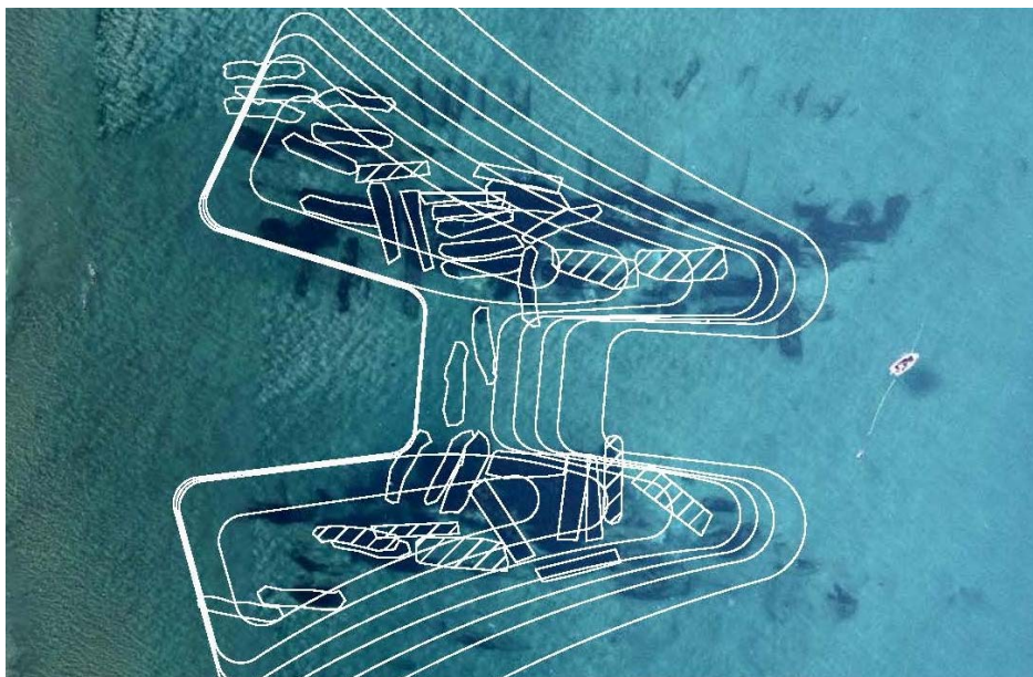
Figure 7. Overlay of July 2011 Aerial Photo with containers placed during maintenance campaigns (ICM)
