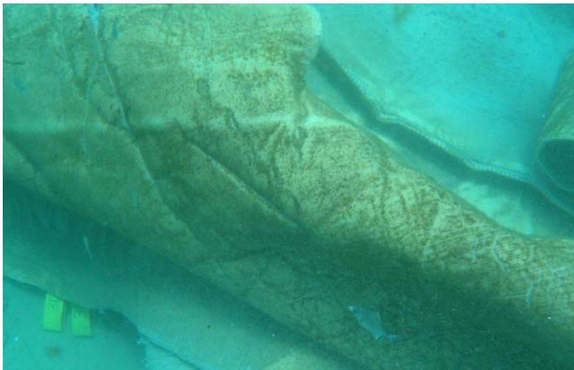
Figure 8. Failed container with polyurethane coating
