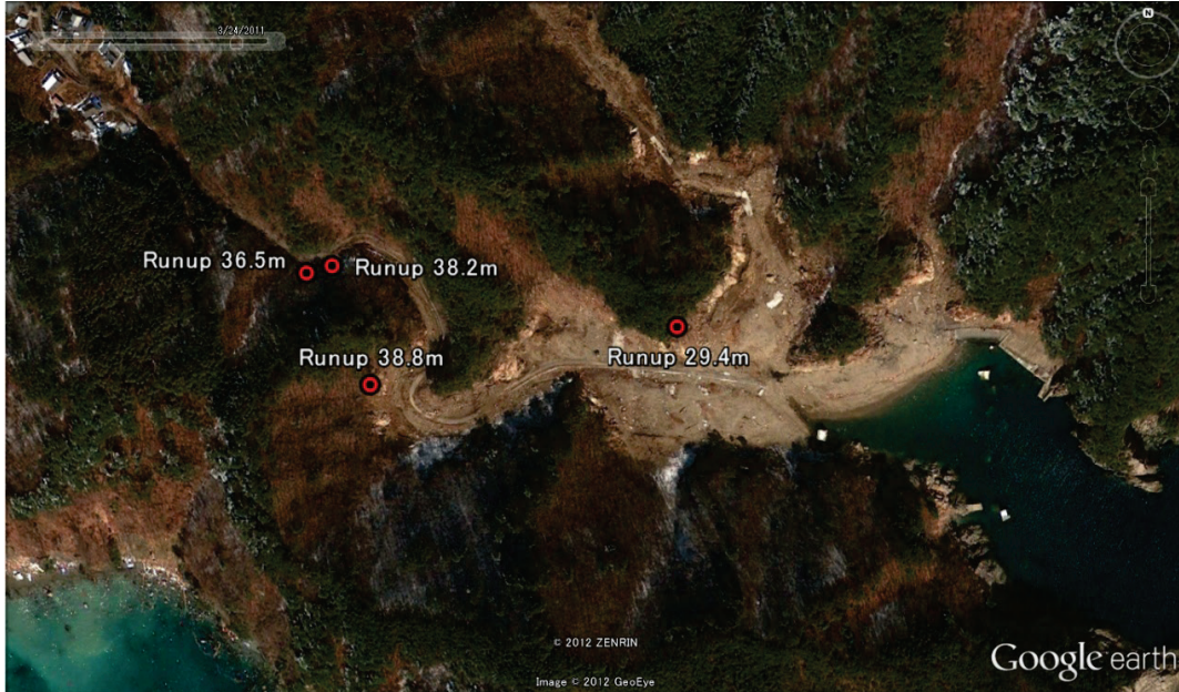
Figure 3. Satellite image of Aneyoshi Valley (Image processed by Google Earth). The markers show measured tsunami heights. The houses at the upper-left corner form Aneyoshi Village which had been relocated to the present location after Showa Sanriku Tsunami in 1933.
