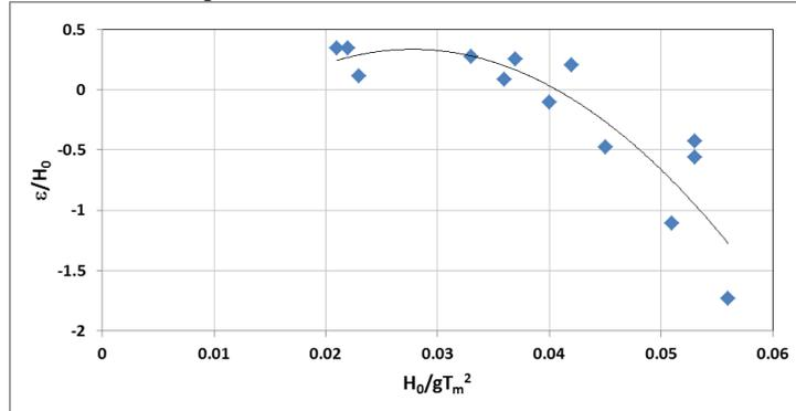
Figure 7 Dimensionless toe level variation against the wave steepness for 1:5 slope and for location  $X=20\text{cm}$
