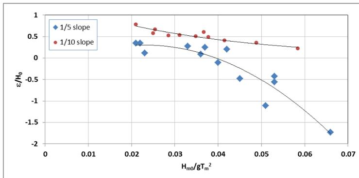
Figure 8 Dimensionless toe level against the wave steepness for both slopes and  $X=20\text{cm}$
