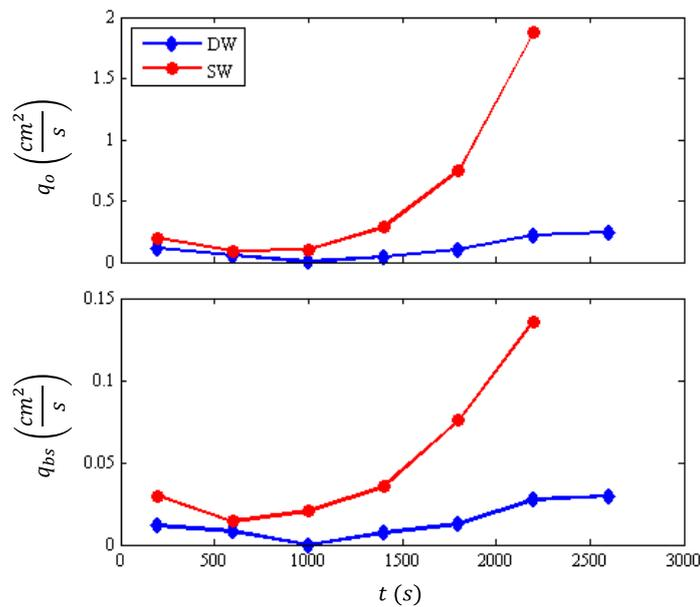
Figure 12. Temporal variations of wave overtopping rate  $q_o$  (top) and sand overwash rate  $q_{bs}$  (bottom) during the DW and SW tests.
