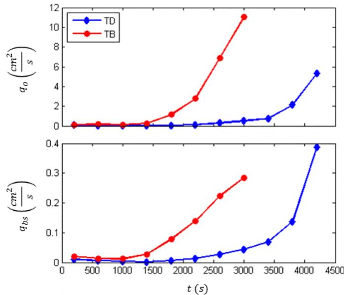
Figure 17. Temporal variations of wave overtopping rate  $q_o$  (top) and sand overwash rate  $q_{bs}$  (bottom) during the TD and TB tests.
