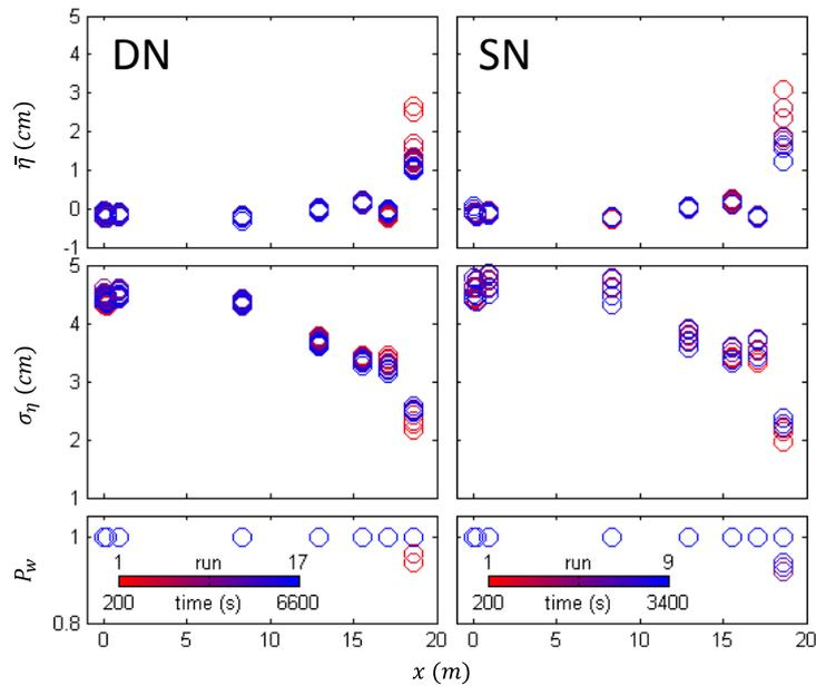
Figure 7. Cross-shore variations of the mean (top), standard deviation (middle) of the free surface elevation and wet probability (bottom) during the DN (left) and SN (right) tests.
