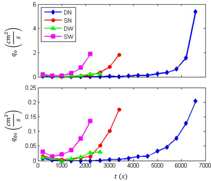
Figure 18. Temporal variations of wave overtopping rate  $q_o$  (top) and sand overwash rate  $q_{bs}$  (bottom) for the DN, SN, DW and SW tests.
