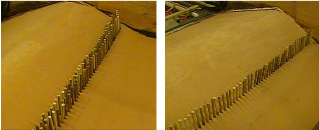
Figure 3. Pile fence configurations before the DN (left) and SN (right) tests.
