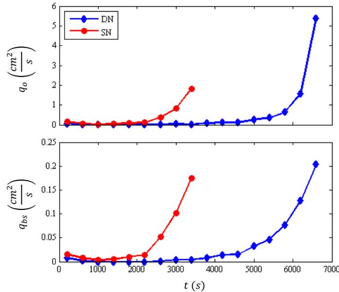
Figure 9. Temporal variations of wave overtopping rate  $q_o$  (top) and sand overwash rate  $q_{bs}$  (bottom) during the DN and SN tests.
