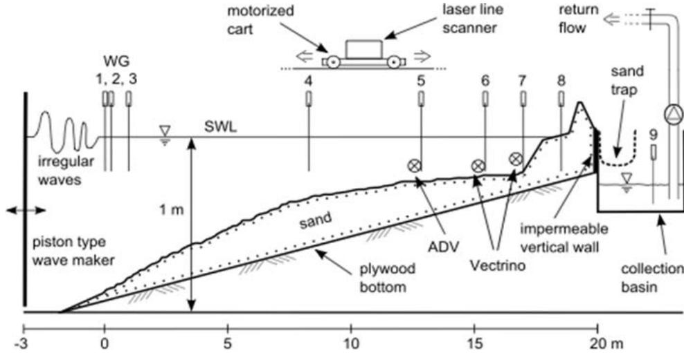
Figure 1. Schematic side view of the experimental setup including wave paddle, sandy beach profile on top of plywood slope, collection basin including sediment trap, water recirculation system, and laser line scanner mounted on a motorized card and location of the instruments measuring the hydrodynamics.
