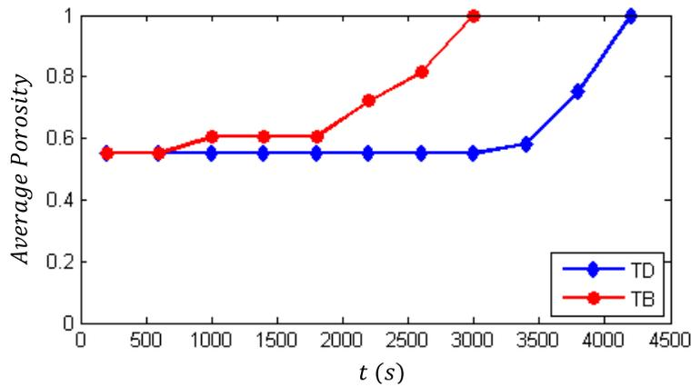
Figure 15. Temporal change in average porosity for the TD and TB tests.
