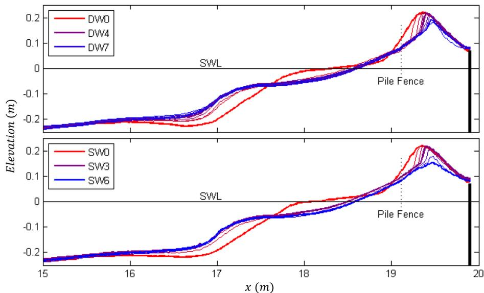
**Figure 11.** Dune profile evolution for DW (top) and SW (bottom) tests. The color scale from red (initial profile) to blue (final profile) indicates the measured profile number (DW: 0-7; SW: 0-6).
