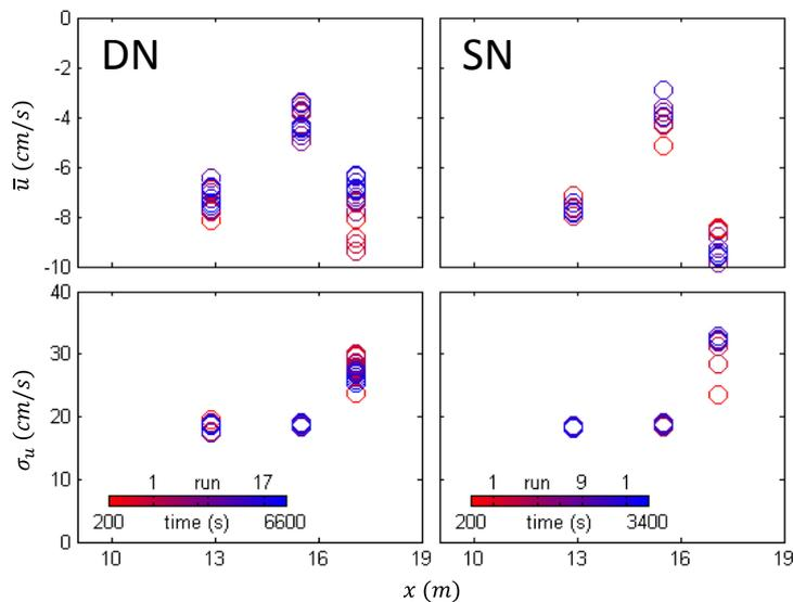
Figure 8. Temporal variations of the mean (top) and standard deviation (bottom) of the cross-shore velocity at the three velocimeters during the DN (left) and SN (right) tests.
