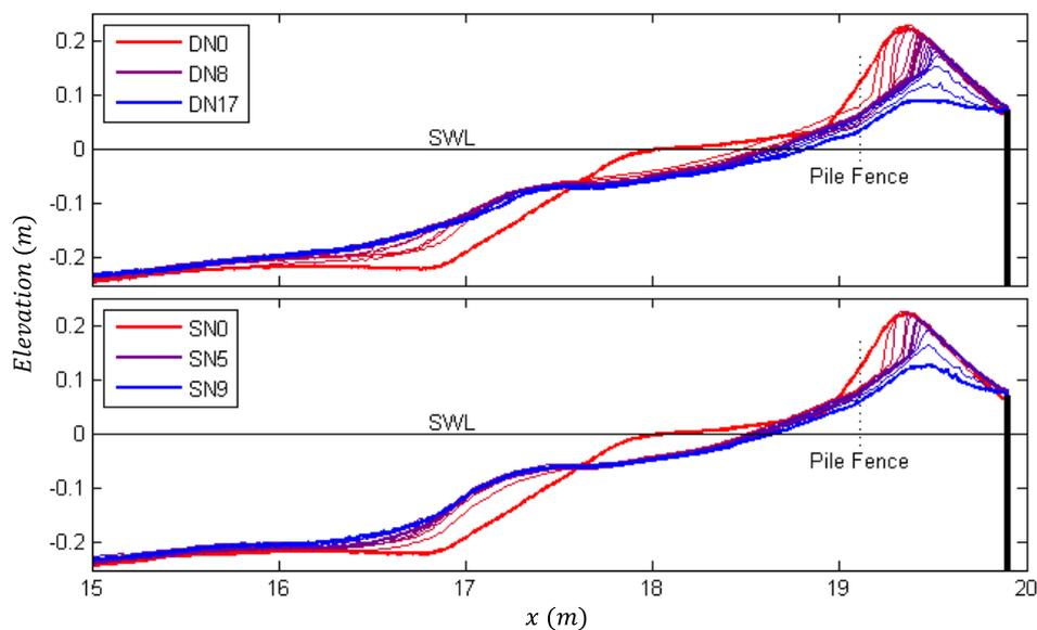
**Figure 6. Dune profile evolution for DN (top) and SN (bottom) tests. The color scale from red (initial profile) to blue (final profile) indicates the measured profile number (DN: 0–17; SN: 0–9).**
