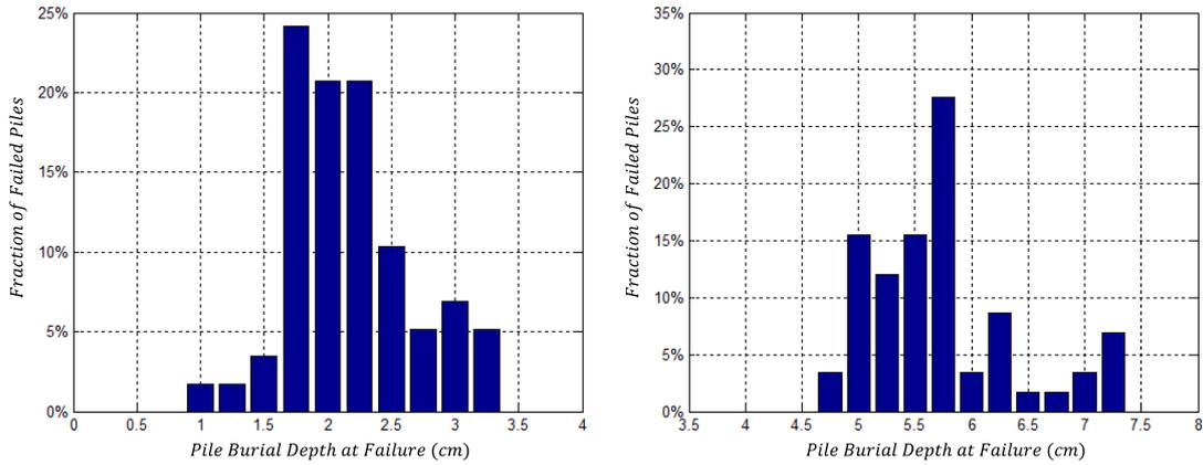
Figure 16. Pile burial depth at failure for the TD (left) and TB (right) test.
