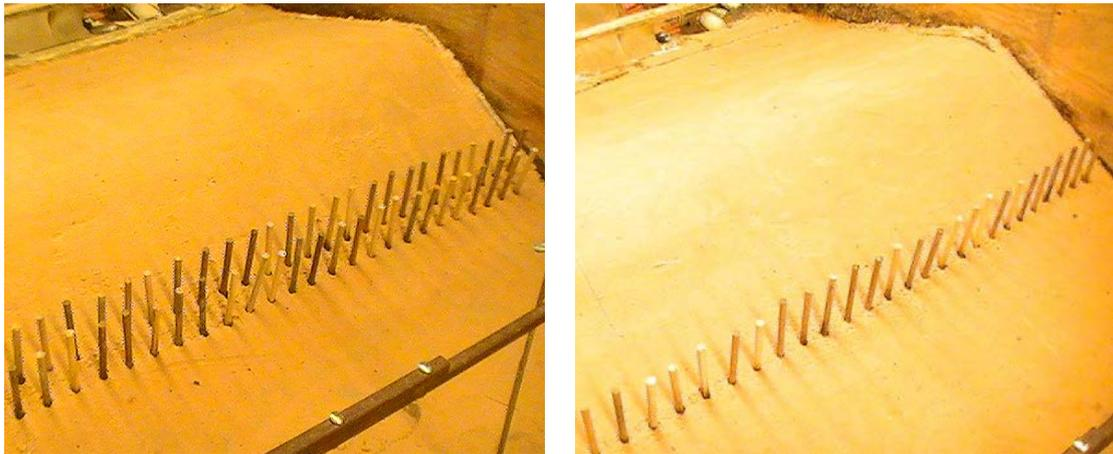
Figure 4. Pile fence configurations before the DW (left) and SW (right) tests.
