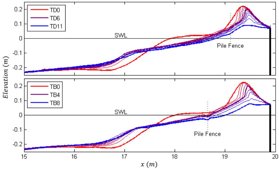
Figure 14. Dune profile evolution for TD (top) and TB (bottom) tests. The color scale from red (initial profile) to blue (final profile) indicates the measured profile number (TD: 0–11; TB: 0–8).
