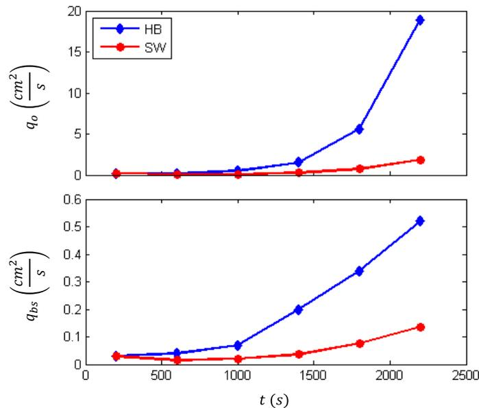
Figure 19. Temporal variations of wave overtopping rate  $q_o$  (top) and sand overwash rate  $q_{bs}$  (bottom) during the HB and SW tests.
