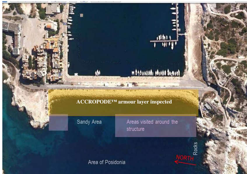
Figure 12. Inspected areas on the Le Frioul breakwater.
