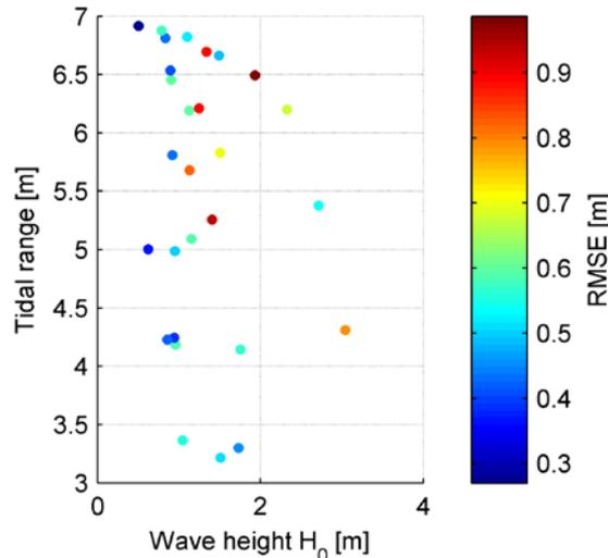
**Figure 3.** The root-mean-square error calculated over the covered inter-tidal area at Porthtowan depending on corresponding tidal range and offshore wave height over a period from July to September.
