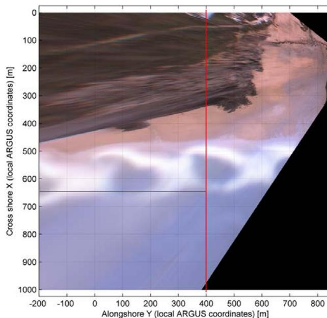
**Figure 9.** Rectified ARGUS timex image at Porthtowan on 20 September 2013 at low tide (WL = -2.85 meters). Offshore is in the bottom of the plot and north is to the left. The red line represents the alongshore position of the cross shore profile as presented in Figure 7. The black line points out the approximate cross shore position of the sub-tidal bar.
