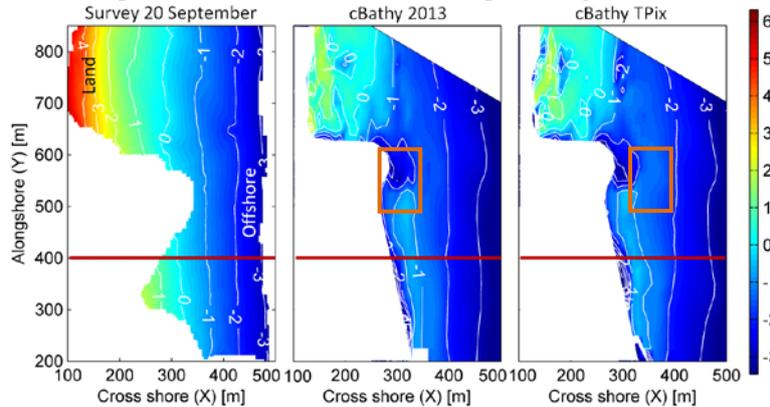
**Figure 6.** On the left hand side the Loess interpolated topographic survey (20 September 2013) is presented while on the right two bathymetry estimates using cBathy 2013 code (in the middle) and on the right side the TPix modification is used. The red squares indicate an area on the cliff face or close to the cliff that passes the quality controls that neither represents a realistic topography nor wave celerity based depth estimations and can be a result of a tile boundary process.
