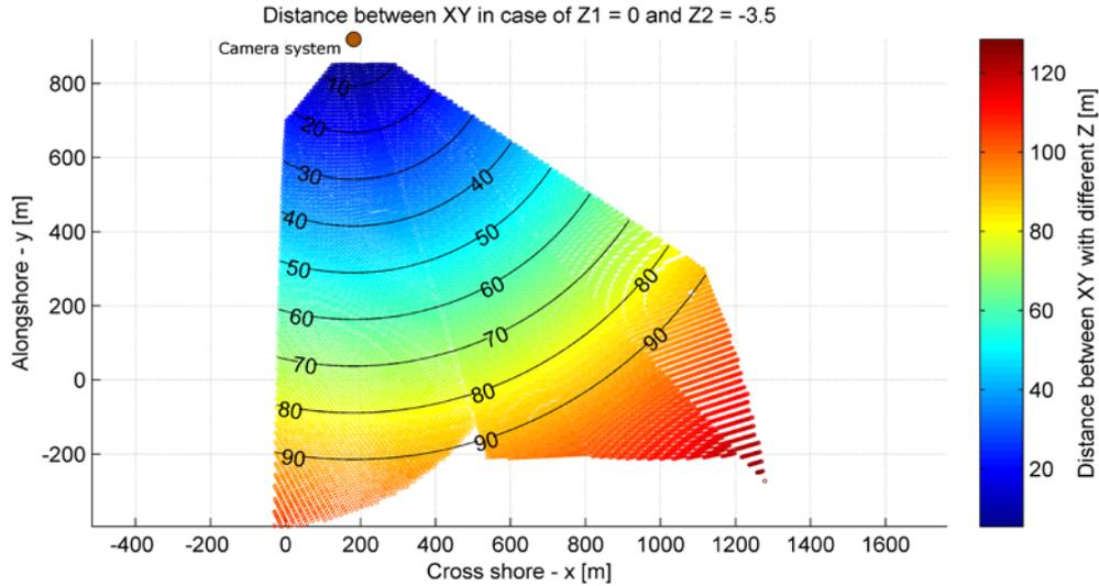
**Figure 5. Representation of the distance (horizontal shift) between the locations at mid ( $Z = 0$  meters) and low tide ( $Z = -3.5$  meters) for the same pixel. Close to the camera (upper part of the figure at  $X, Y = 181.5\text{m}, 919\text{m}$ ) the horizontal shift is limited while further away from the camera the distance between the high and low tide position of a pixel up to 128 meters.**
