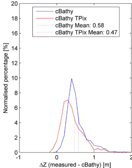
**Figure 8. Distribution of the difference ( $\Delta Z$ ) between the survey and the cBathy bathymetry estimations over the whole survey domain for 20 September 2013 (spring tide). The mean of  $\Delta Z$  for the TPix implementation (0.47 meters) is ~18.9% smaller in the inter-tidal zone compared to the 2013 cBathy code (0.58 meters). In terms of standard deviation the original 2013 cBathy code is smaller (0.28 meters) while the spreading for the TPix implementation is larger (0.32 meters).**
