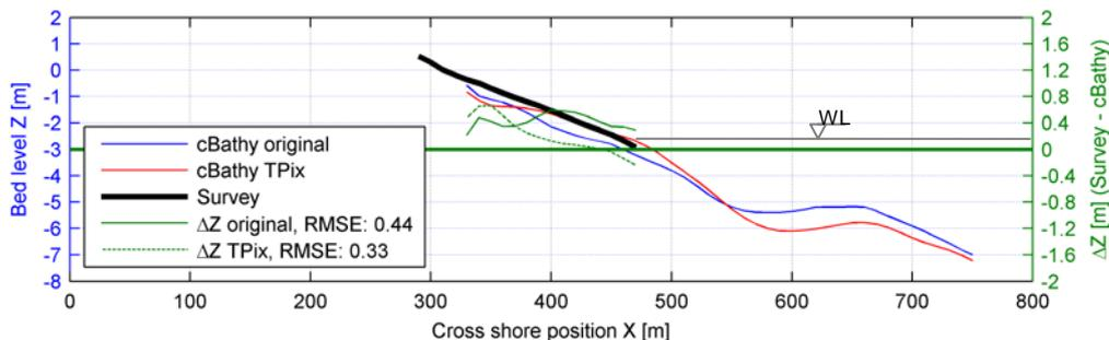
**Figure 7.** Cross shore cross section of the estimated beach profiles (blue lines), beach survey (black line) and comparison between the beach survey and the estimated bathymetry (green lines). The collected survey data is Loess interpolated as well as the Kalman results of the depth estimates. The grey line represents the water level at low water.
