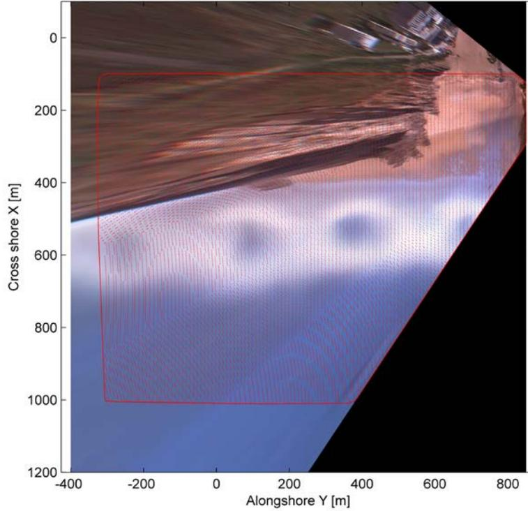
**Figure 2. A rectified merged ARGUS timex image at Porthtowan utilising four cameras. The red line indicates the boundaries of the user defined pixel stacking area and the small dots represent the actual pixel stack location. The stretched pixels on the cliff face (100 to 400 metres in X and -300 to 400 metres alongshore) are excluded from the cBathy analysis.**
