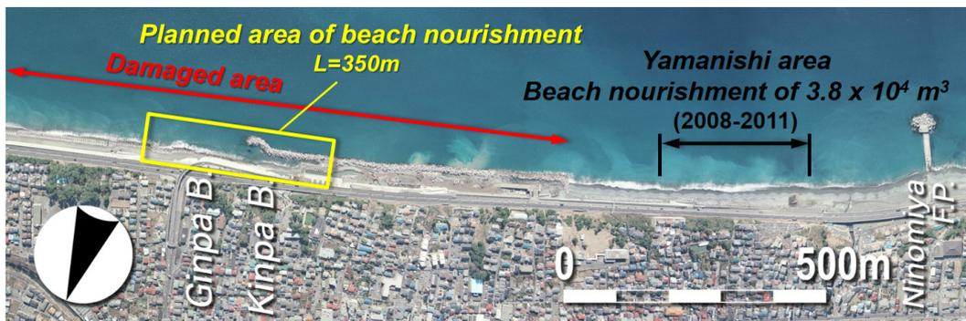
Fig. 4. Location of Yamanishi area where beach nourishment using coarse materials was carried out.
