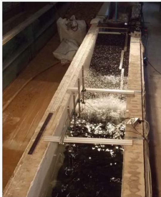
Figure 4. Configuration c1 under wave attack in the 1m wave flume of the LWI.
