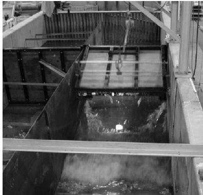
Figure 4. Physical model impoundment reservoir and gate
