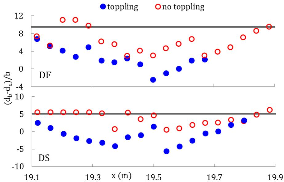
Figure 10. Burial depth ( $d_b-d_e$ ) normalized by dowel diameter  $b$  before and after toppling run for DF and DS tests.
