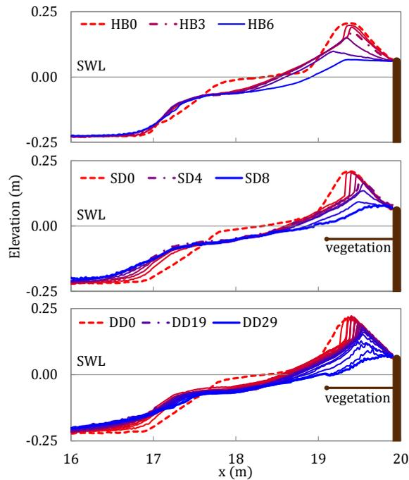
Figure 3. Measured dune profiles for HB, SD and DD tests.
