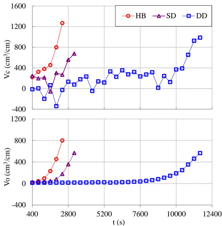
Figure 5. Temporal variations of cumulative sand volume change  $V_c$  and overwash volume  $V_o$  per unit width for HB, SD and DD tests.
