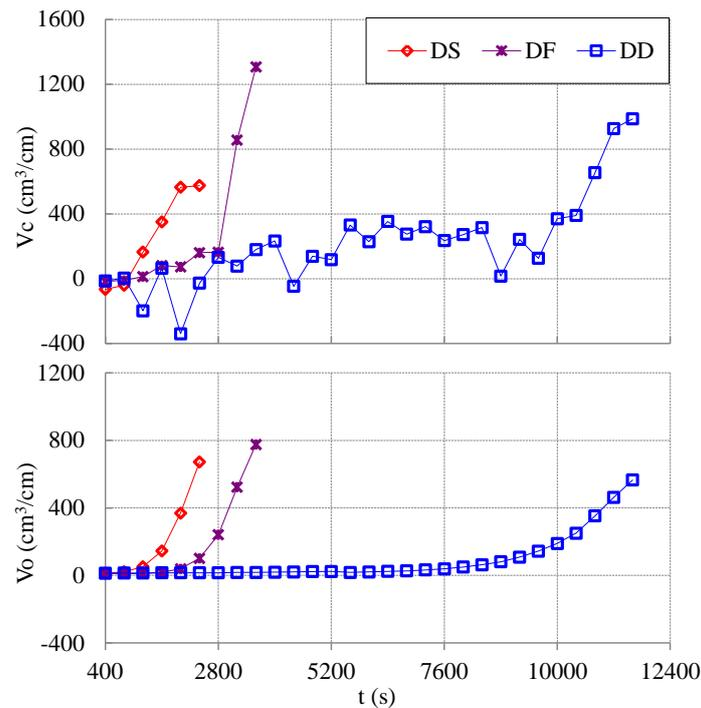
**Figure 9.** Temporal variations of cumulative sand volume change  $V_c$  and overwash volume  $V_o$  per unit width for DD, DF and DS tests.
