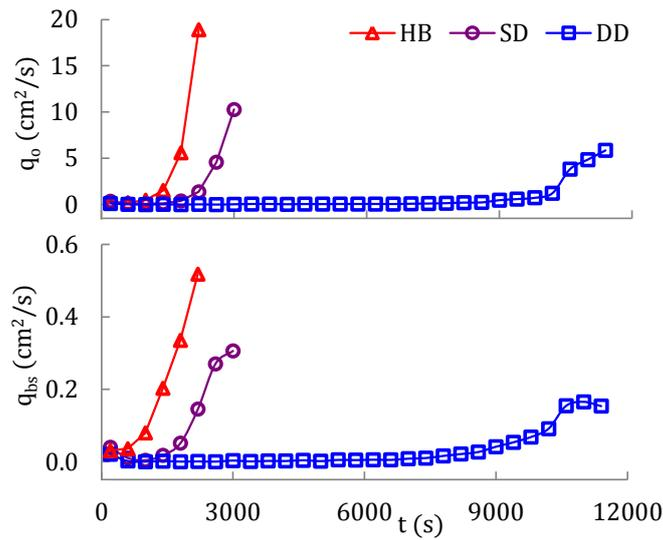
Figure 4. Temporal variations of wave overtopping rate  $q_o$  and sand overwash rate  $q_{bs}$  for HB, SD and DD tests.
