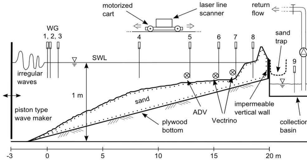
**Figure 1. Schematic view of the experimental set-up including wave paddle, sandy beach profile on top of plywood slope, collection basin including sediment trap, water recirculation system, laser line scanner mounted to a motorized cart and location of the instruments measuring the hydrodynamics with a dune profile without wooden dowels.**
