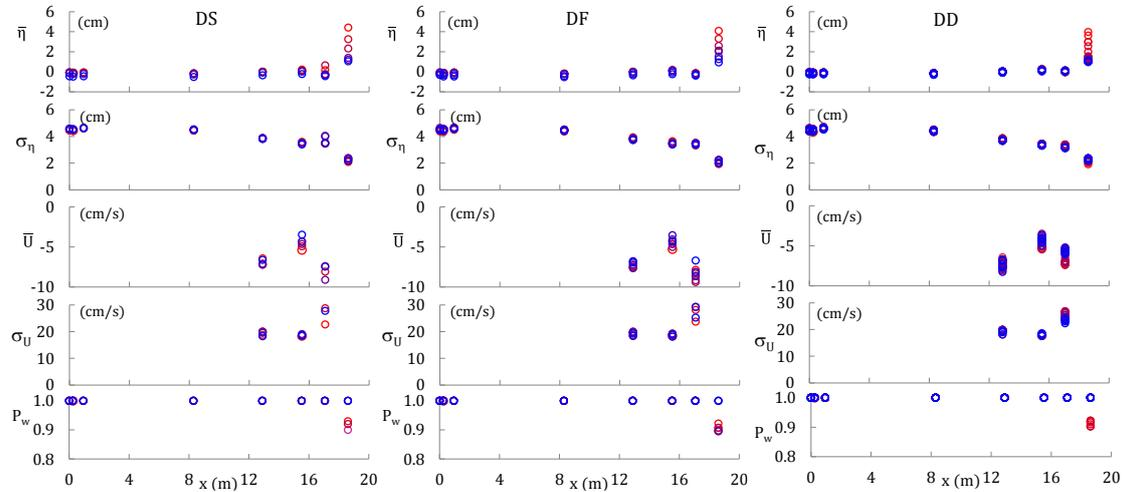
**Figure 6. Measured mean and standard deviation of free surface elevation and cross-shore velocity together with wet probability  $P_w$  for DS, DF and DD tests.**
