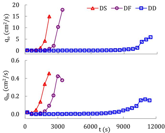
Figure 8. Temporal variations of wave overtopping rate  $q_o$  and sand overwash rate  $q_{bs}$  for DD, DF and DS tests.
