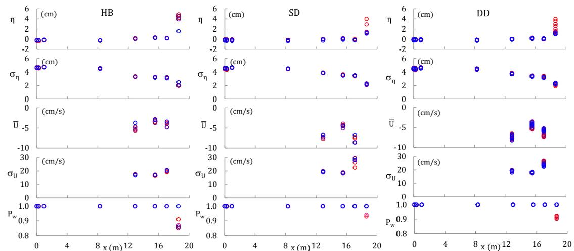
Figure 2. Measured mean and standard derivation of free surface elevation and cross-shore velocity together with wet probability  $P_w$  for HB, SD and DD tests.
