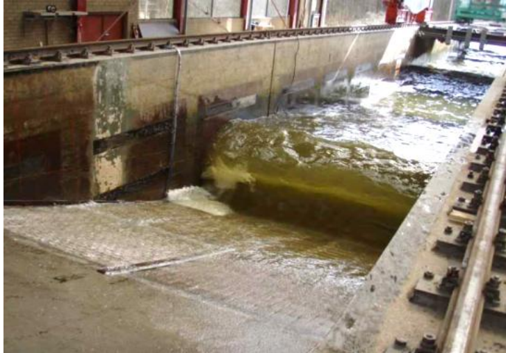
Figure 16, Wave attack on test section in Delta flume
