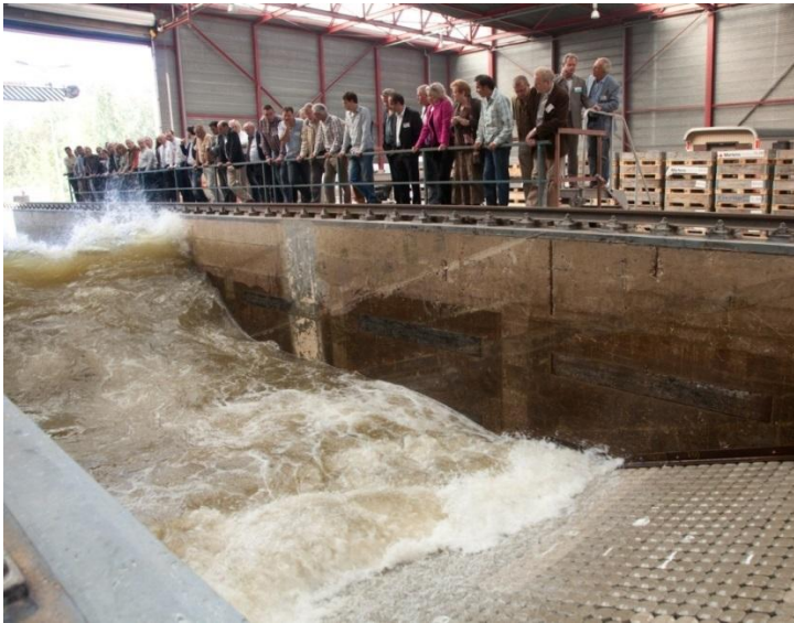
Figure 12. Large-scale tests on a block revetment in the Delta Flume of Deltares.
