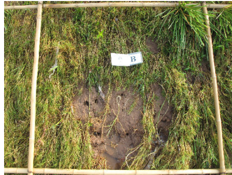
Figure 7: A weak spot on Thai Tho grass slope, the bamboo frame is 1 m × 1 m.
