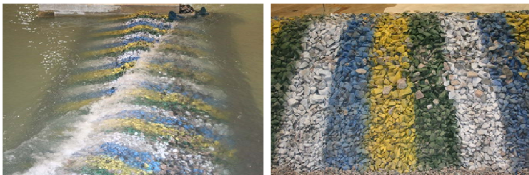
Figure 7. Testing a partly reshaping berm breakwater with severe overtopping (left) and start of damage to the rear (right).
