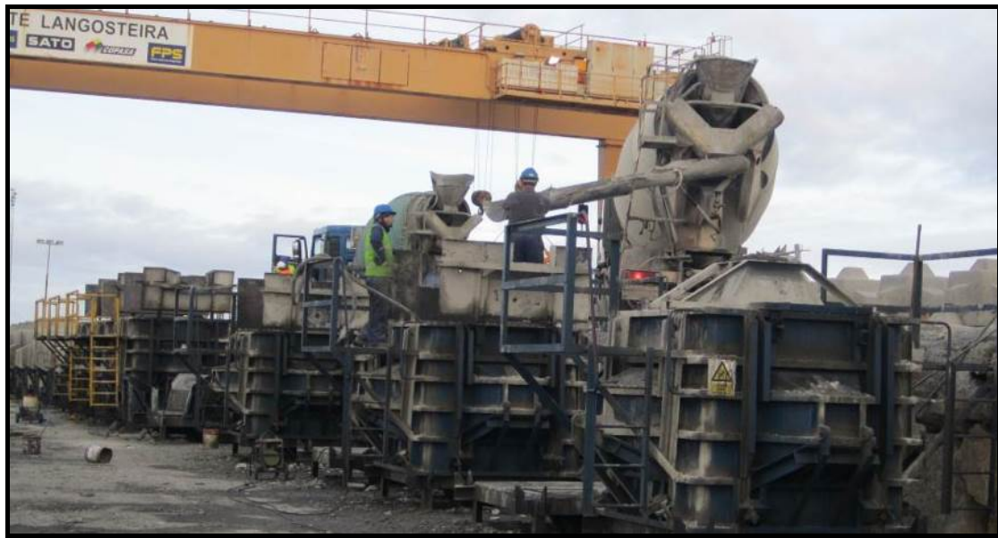
Figure 7. Production line of 25-tonne Cubipod units.
