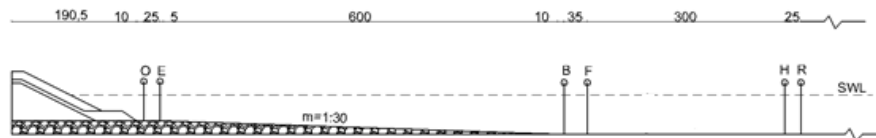
Figure 5: Side View of the Experimental Setup (Dimensions are given in centimeters and figure is not to scale. O, E, B, F, H and R are wave measurement gauges.)
