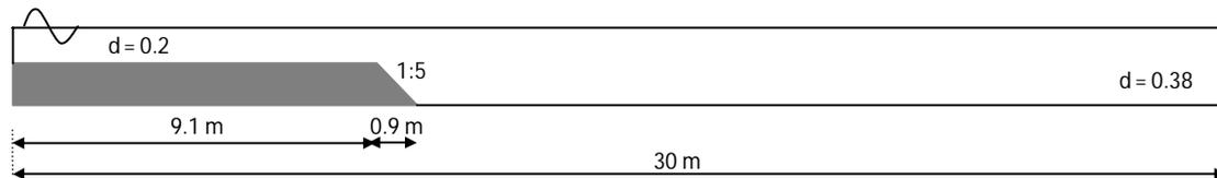
Figure 8: Geometry of down-slope verification cases.
