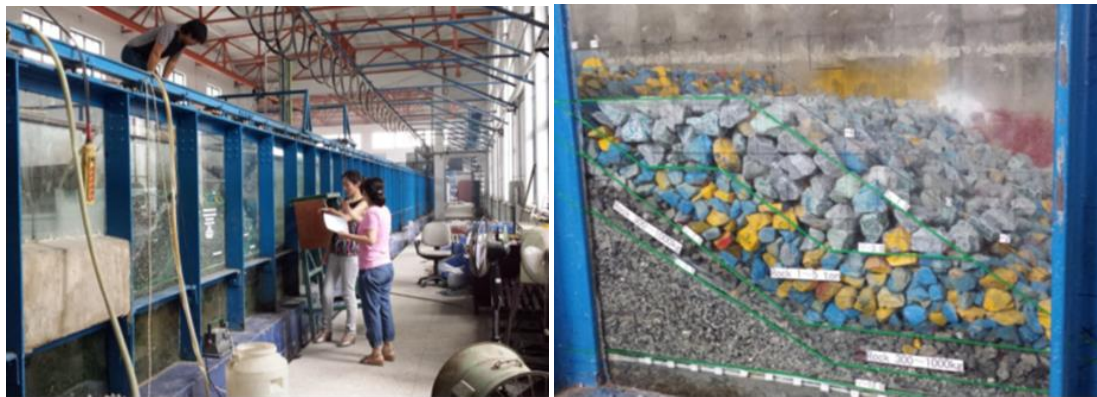
Figure 5. The testing facility in Tianjin Port Engineering Institute, flume and tested cross section.
