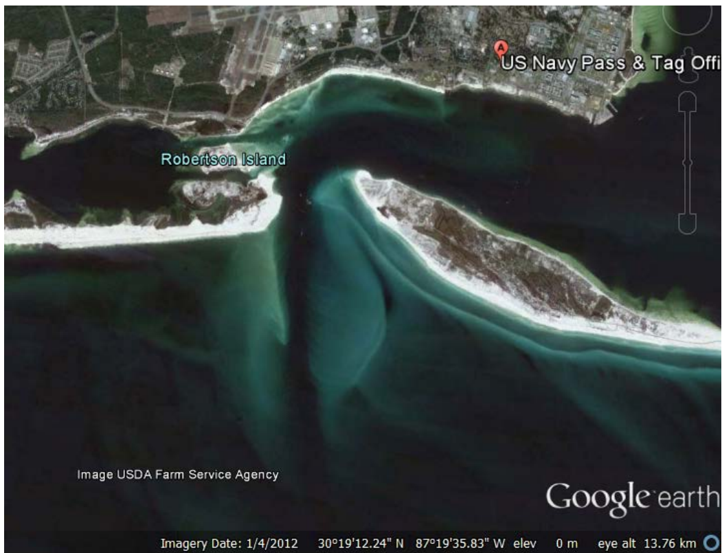
Figure 3: Pensacola Pass on Florida, US near 30°19.5'N 87°18.5'W. The inlet spring tidal prism of P=2.7 \times 10^9 \text{ m}^3 , corresponding to large bay surface area of A_B \approx 477 \text{ km}^2 (FL32399 report, 2012) and mean spring tidal amplitude approximately a_B = 0.27 \text{ m} while average ocean amplitude in this area is a_o = 0.21 \text{ m} . The Bay tide has perfect response to the ocean tide due to large entrance area of the order of 10000 \text{ m}^2 . The average significant wave height is around \bar{H}_s \approx 1 \text{ m} . Two well-developed ebb deltas and large value of \frac{\hat{Q}_{\text{actual}}}{\sqrt{gH_s^5}} = 3029 indicate that the system is tidal dominated estuary while it is wave dominated according to Hayes (1979).
