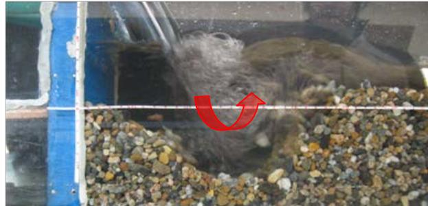
Figure 4 Scouring downstream of over flow
