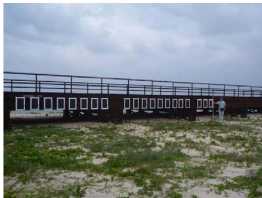
Figure 4. Test pieces of geosynthetic exposed on backshore of Nagayamanohama beach.
