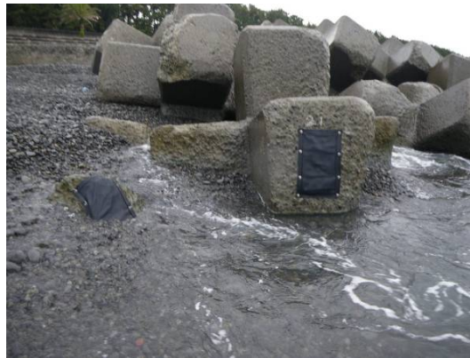
Figure 3. Test pieces of geosynthetic materials attached on the surface of concrete block.
