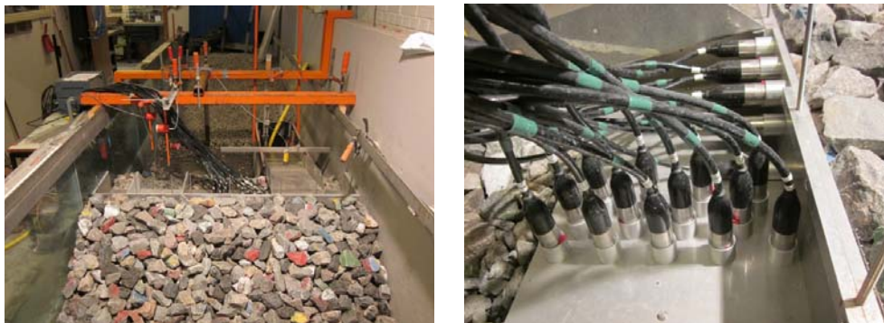
Figure 4. (left) Front view of breakwater, (right) Pressure transducers in fixed part of crown wall. (Nørgaard et al., 2012)
