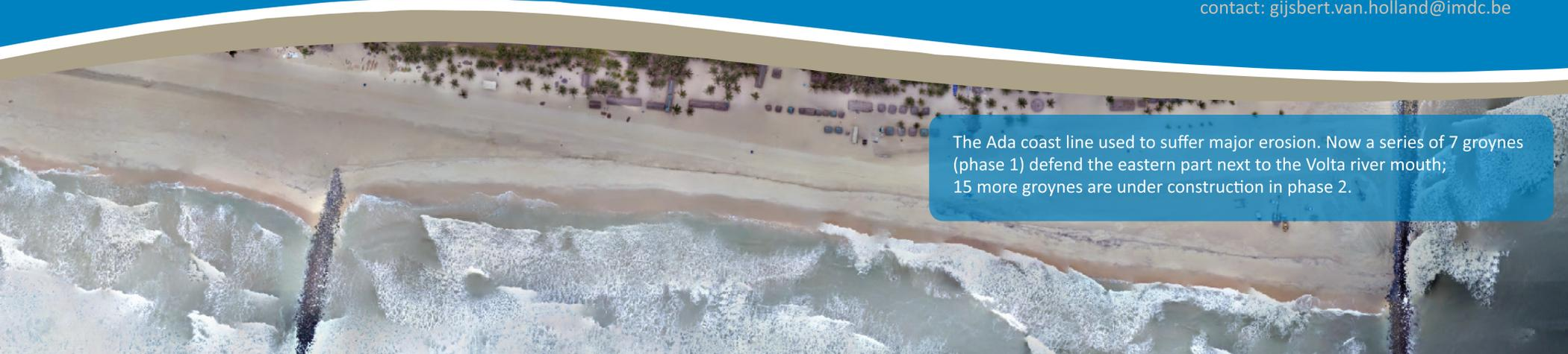
The Ada coast line used to suffer major erosion. Now a series of 7 groynes (phase 1) defend the eastern part next to the Volta river mouth; 15 more groynes are under construction in phase 2.
