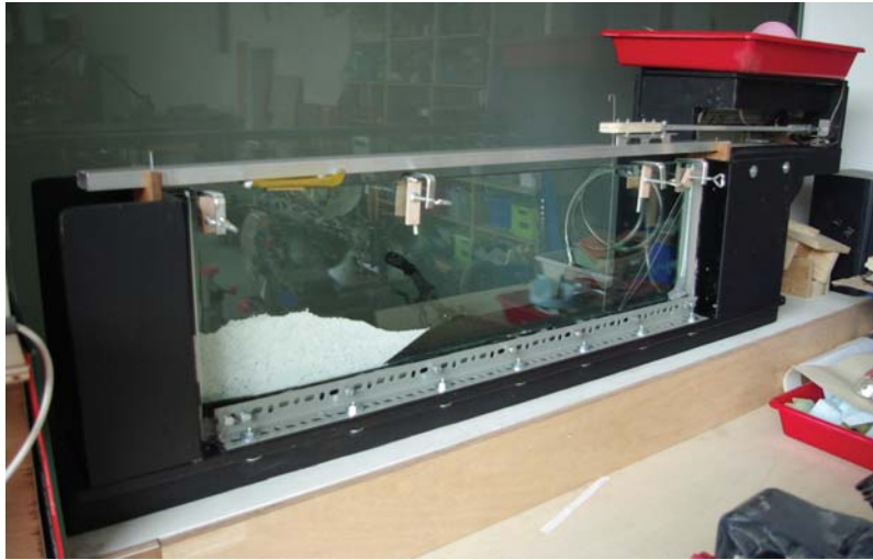
Figure 7: The second, dry Hele-Shaw cell with the linear, programmable motor of a disassembled printer on the right, the black wedge in the middle, white particles, and the clamping system.
