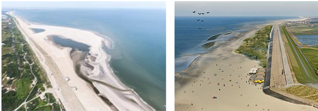
Figure 2. Left: Aerial photograph of the Sand Motor in July 2012 (RWS/Joop van Houdt). Right: Artist impression of the mega-nourishment in front of the sea dike near Petten (Hoogheemraadschap Noorderkwartier, www.kustopkracht.nl ).
