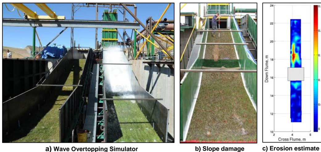
Figure 2. CSU Wave Overtopping Simulator and typical grass cover damage.
