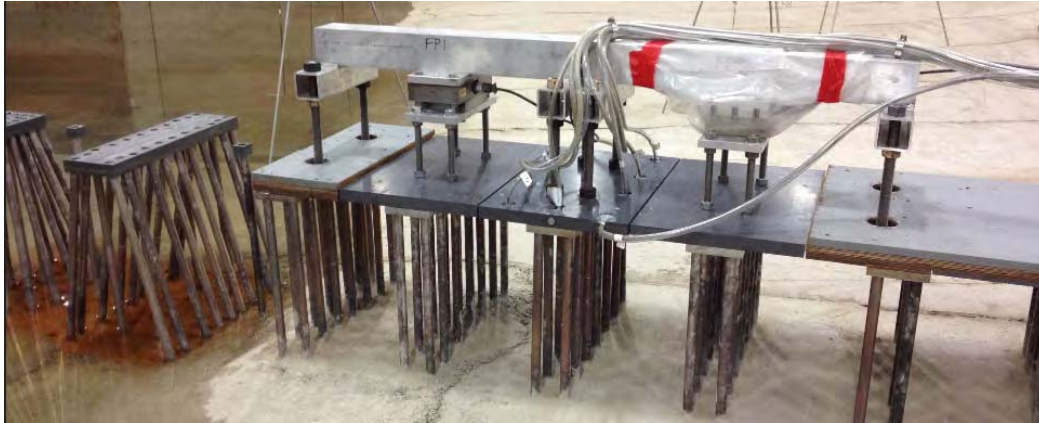
Figure 11. Force-Pressure-Force (FPF) Instrumentation Array on Solid Deck Pier
