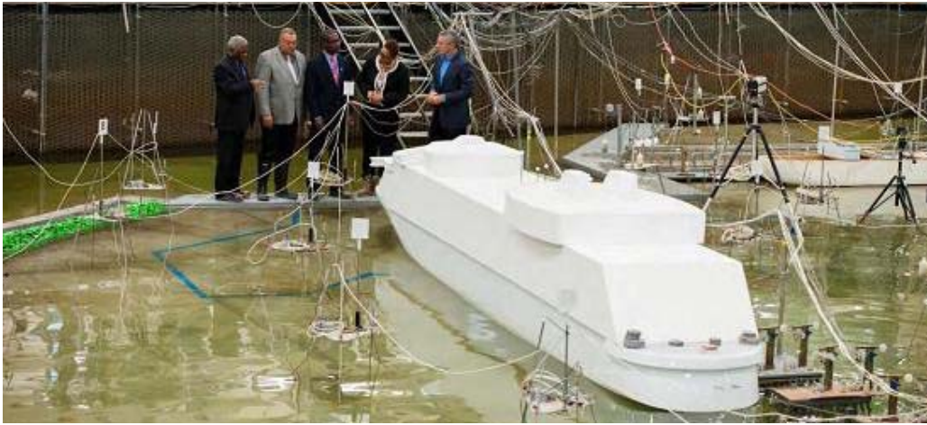
Figure 7. Closeup of Oasis at Berth 1N during Moored Ship Response Tests
