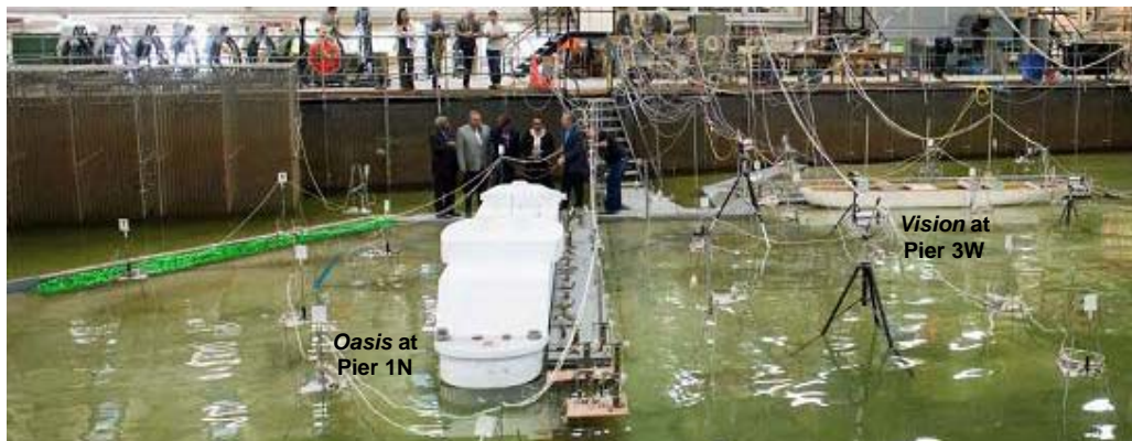
Figure 6. Overview of Physical Model during Moored Ship Response Tests
