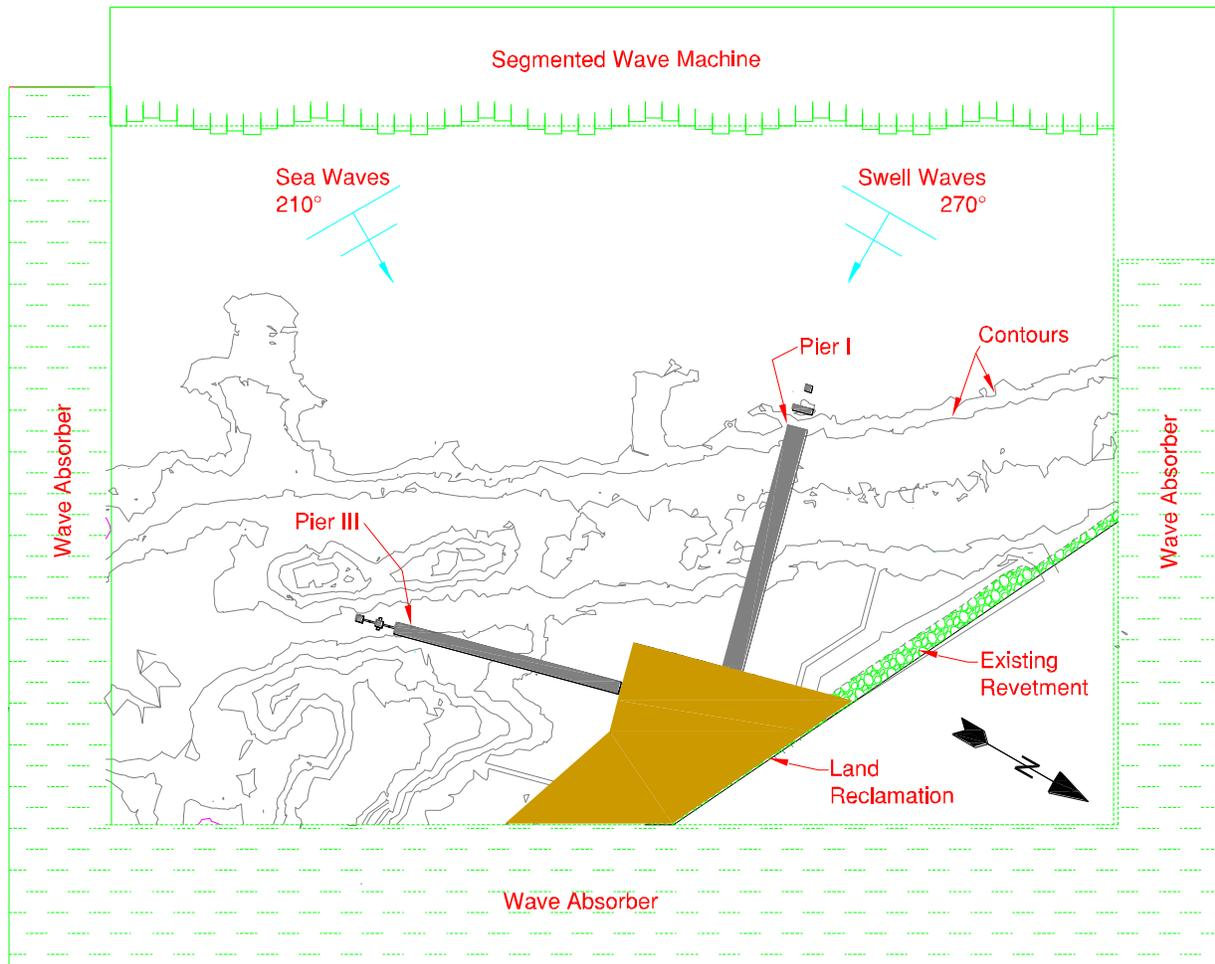
Figure 3: Physical model after bathymetry and port construction.
