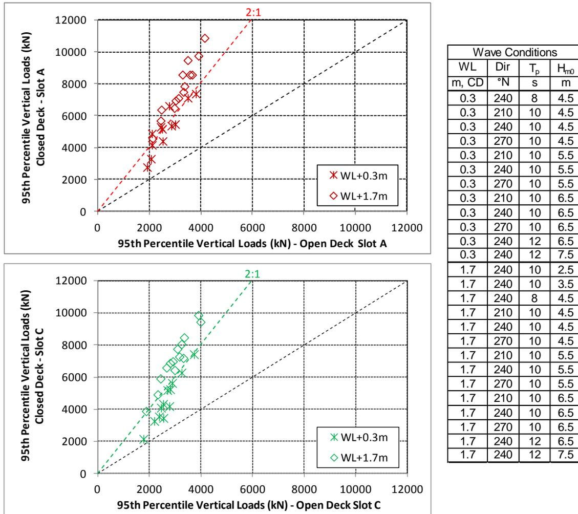
Figure 13: Reduction in peak uplift loads for the semi-open deck structure: a) force panel A; b) force panel C.
