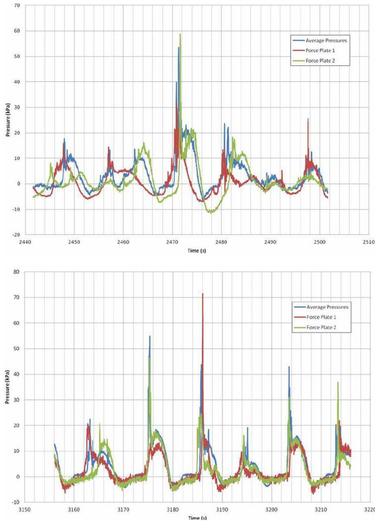
Figure 12: Example time series of spatially averaged uplift pressure from the F-P-F panels: a) the outer end of Pier I; b) the outer end of Pier III.
