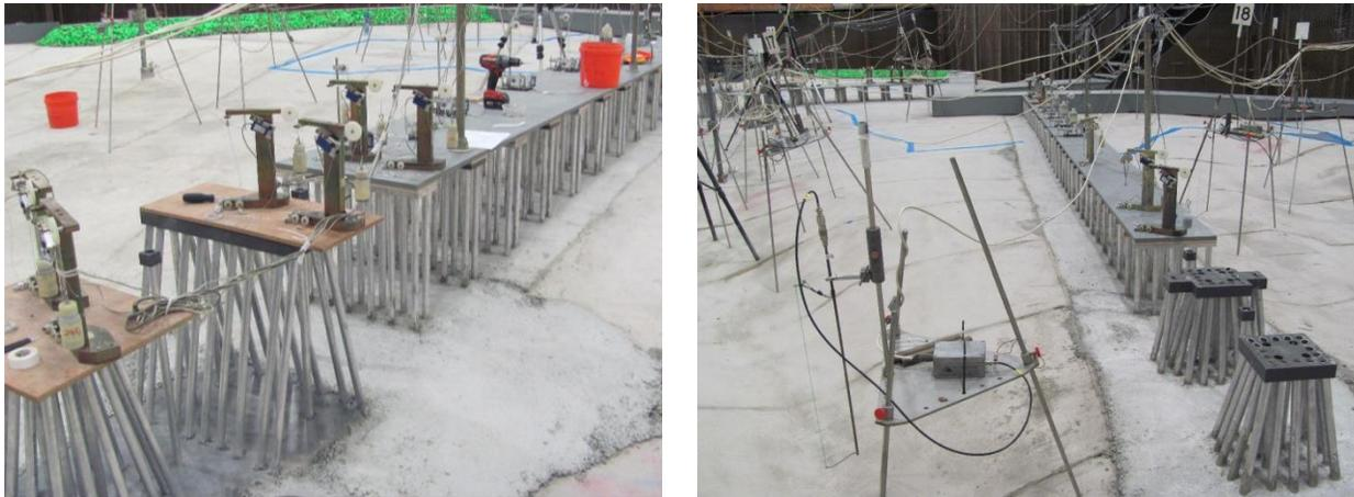
The reactions at each fender and the tension loads in all mooring lines were measured continuously during the study and compared with safe working limits. Tests were conducted with both vessels moored at their berths simultaneously, the Oasis at Pier I and the Grandeur at Pier III. Additional tests were performed with the Grandeur moored at Pier I and the Oasis removed from the physical model.
