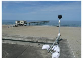
Picture 1. A research facility (HORS) and a sound pressure level meter.
