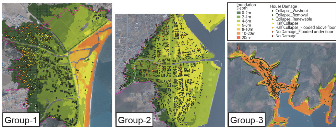
Figure 13. Examples of spatial distribution of inundation area, inundation depth and house damage of each group.
