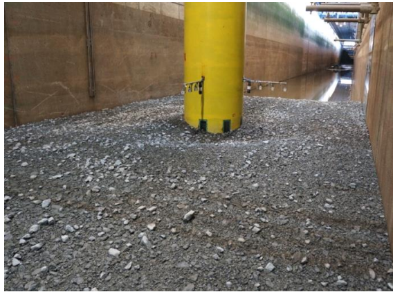
Figure 4: Final scour development around the monopile after 9000 waves and maximum significant wave height H_s = 1.3 m. Waves are propagating in the direction of view.
