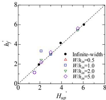
Figure 8. Relationship between the non-dimensional specific energy and the non-dimensional water level in the front of a structure
