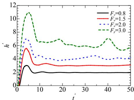
Figure 2. Time-history of the water level in front of a structure in infinite-width structure case
