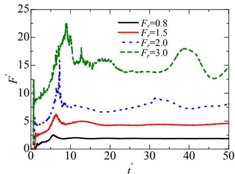
Figure 3. Time-history of the hydrodynamic force acting on the front face of a structure in infinite-width structure case
