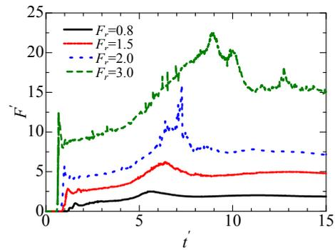
Figure 5. Time-history of the hydrodynamic force acting on a front face of structure in infinite-width structure case between  $t=0$  and  $t=15$
