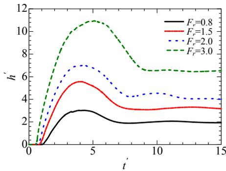
Figure 4. Time-history of the water level in front of a structure in infinite-width structure case between  $t=0$  and  $t=15$
