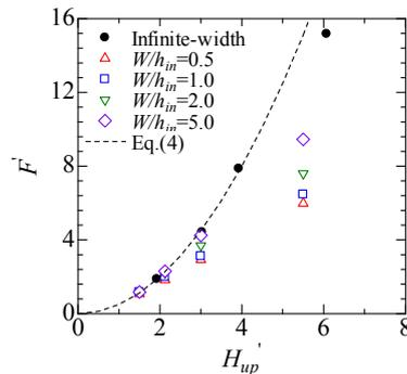
Figure 9. Relationship between the non-dimensional specific energy and the non-dimensional quasi-steady force acting of the front face of a structure
