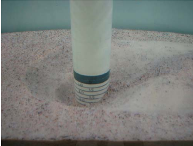
Figure 1. Calibrated pile in the small flume
