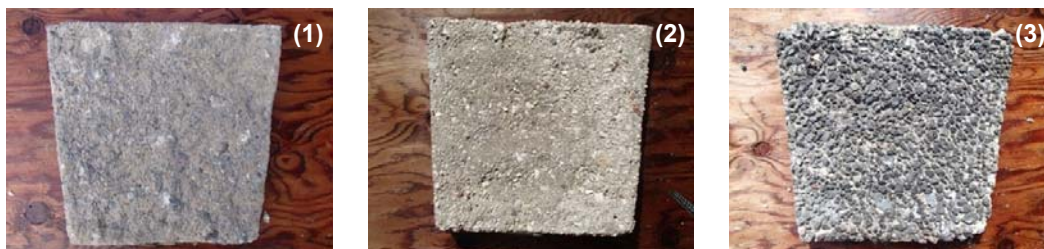
Figure 1. Three concrete test plate types were made with the same mix design and used (1) basalt, (2) limestone, and (3) recycled concrete/asphalt aggregate materials.
