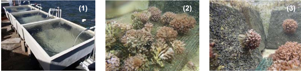
Figure 2. (1) Concrete plates were deployed in seawater test tanks in the laboratory experimental setup. (2) P. damicornis were placed in the center of each tank, and (3) were also cemented on half of the test plates.
