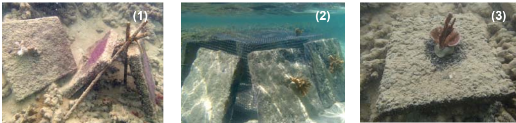
Figure 4. Concrete plates were deployed in plots of six on the sea floor in the field experimental setups at the (1) deep and (2) shallow sites. (3) M. capitata were cemented on half the test plates.
