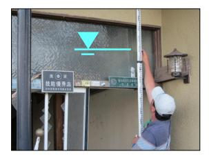
Figure 4. Measurement of tsunami inundation height
