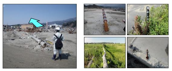
Figure 2. Measurement of tsunami flow direction (left) and examples of pillar-shaped object (right)
