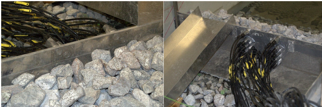
Figure 3: Crown wall with pressure transducers.
