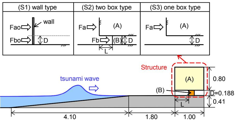
Figure 3. Set up of experiments (unit: m).
