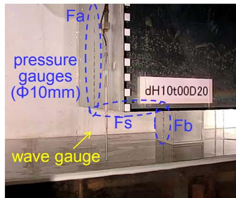
Photo 2. Configuration of the gauges
