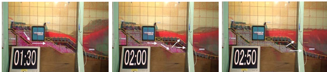
Photo 4. Flow motions of overtopping water
