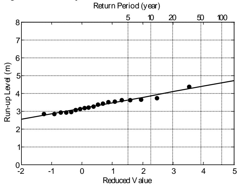
Figure 6. Extrapolated linear fit based on a Gumbel distribution for return periods of annual maximum runup level, 1993-2011. Empirical distribution function (black dots) estimated with the Gringorten plotting position formula.
