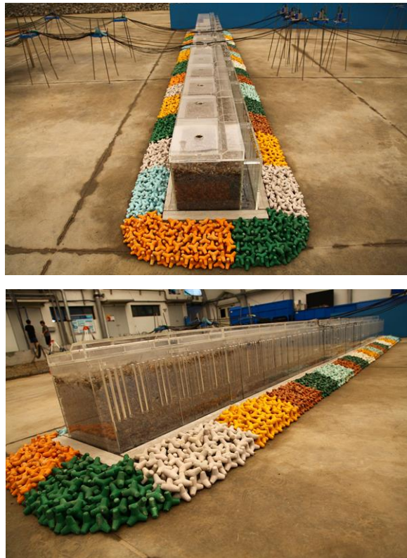
Figure 2. Side and corner views of the perforated caisson installed in the wave basin.
