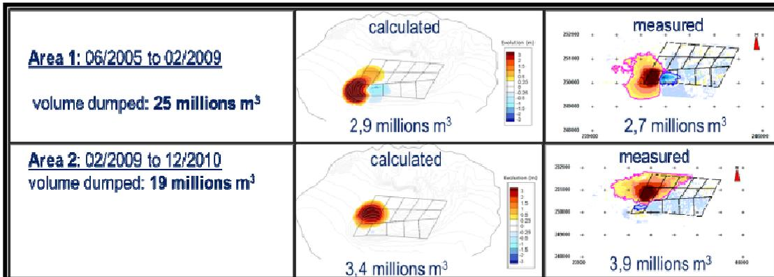
Figure 17: Bathymetry evolution
