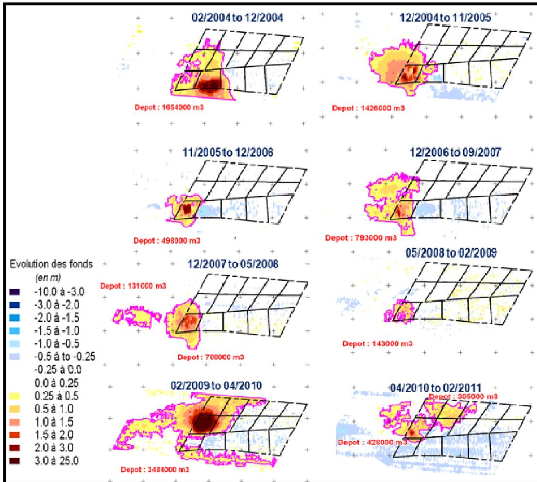
Figure 8: Evolution of Bathymetry
