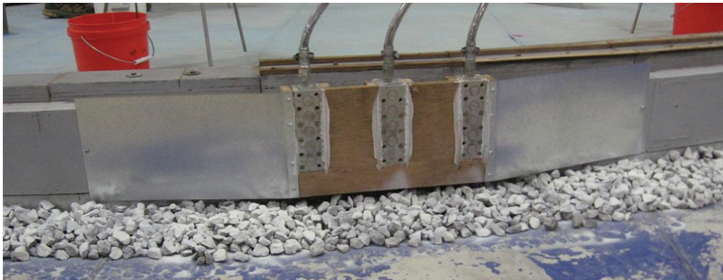
Figure 12. Array of pressure sensors on the seaward face of the model breakwater.
