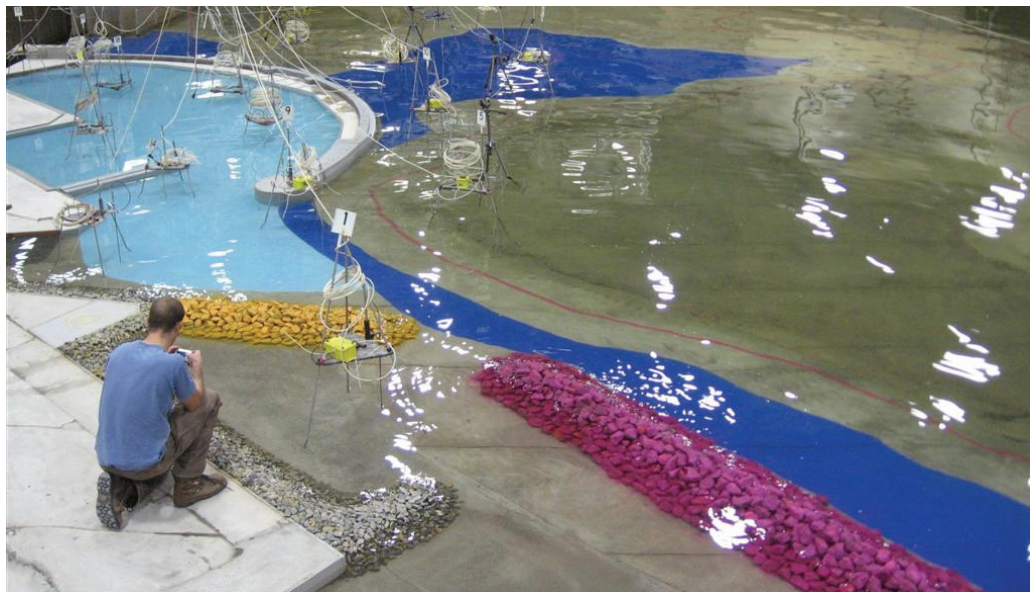
Figure 3. Physical model of the proposed mega-yacht marina.
