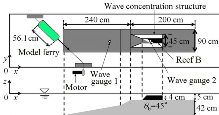
Figure 9. Schematic of laboratory setup. The scale of length is 1/100. The upper and lower figures show the plan and side views, respectively. The wave concentration structures are not drawn in the side view.
