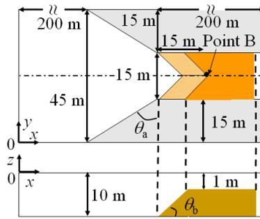
Figure 3. Wave concentration structures and Reef A.
