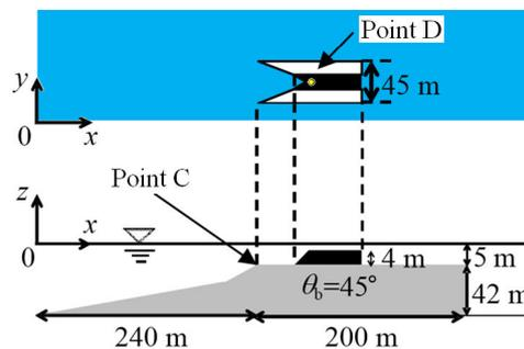
Figure 7. Seabed configuration and wave concentration structures with Reef A utilized in the numerical computation. The upper and lower figures show the plan and side views, respectively. The wave concentration structures are not drawn in the side view.
