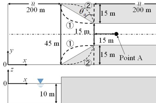
Figure 2. Wave concentration structures. The upper and lower figures show the plan and side views, respectively.
