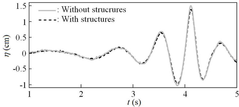
(a) Water surface displacements at the location of Wave gauge 1
