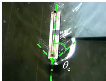
Figure 10. Model-ferry generated waves.
