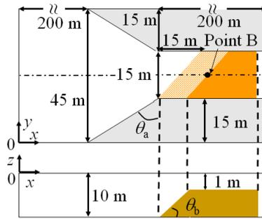
Figure 4. Wave concentration structures and Reef B.
