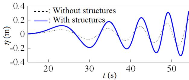
Figure 8. Numerical calculation results of water surface displacements at Point D shown in Fig. 7, in the cases with and without the wave concentration structures and Reef A.
