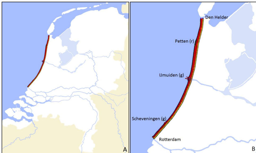
Figure 5. Schematic overview of (A) the Holland coast in relation to the Netherlands and (B) a zoom of the Unibest CL+ model of the Holland coast incl. groynes (Schevevingen & IJmuiden) and revetment (Petten).
