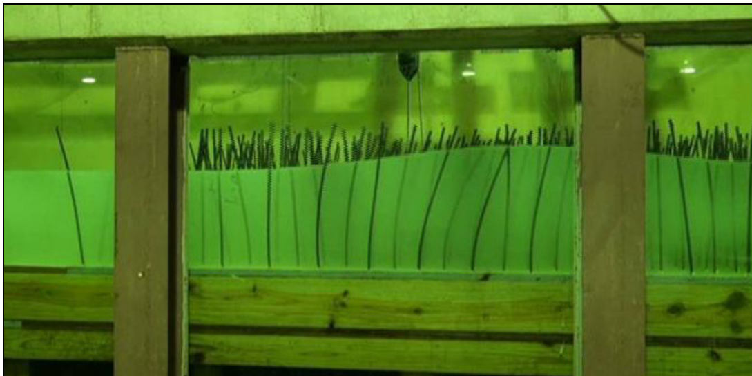
Figure 2. Artificial vegetation under wave action.
